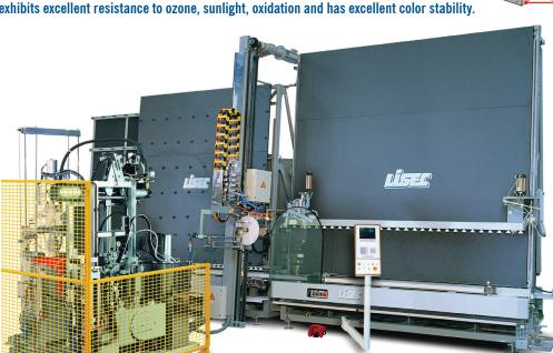
Research proves that insulating glass units manufactured on automated lines have fewer seal failures than manually fabricated IGUs. Hartung Glass Industries currently has six automated insulating glass unit lines.
