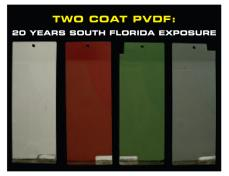
Demonstrating the long-term performance of PVDF coatings treated with a three-coat system with a clear coat after 20 years of South Florida exposure testing.
