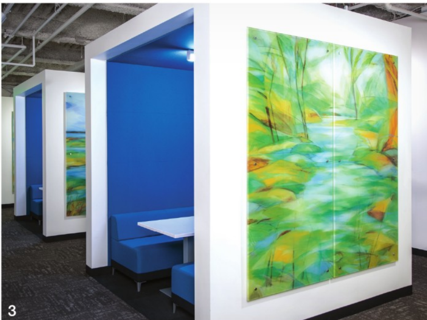
2. The artwork, entitled Alameda County Water , was printed on large glass panels using a Dip-Tech AR4000. Photo Credit: Sibila Savage Photography. 3. Digital images of Norling's watercolor murals were printed onto low-iron Starfire glass panels using a Dip-Tech digital ceramic glass printer. Photo Credit: Sibila Savage Photography.
